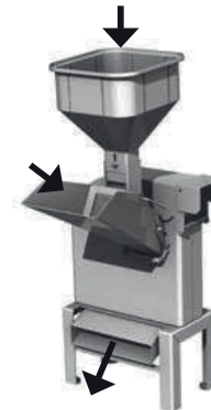
The product is placed in the intake chute or hopper and comes out from the lower chute.
